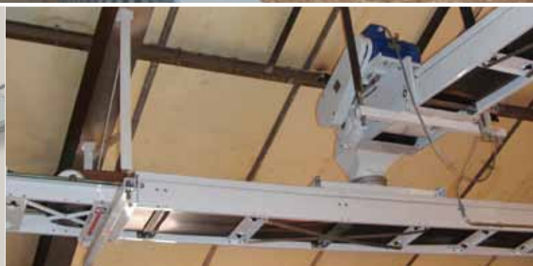
Solution with two belts fitted at a 90° angle. The lower conveyor belt can move lengthwise.
