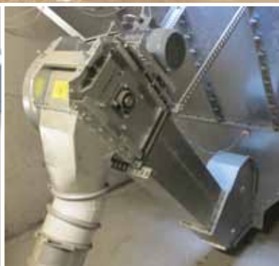
Chain elevator with 45° angle. Drive section with belt drive
