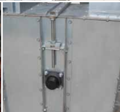
Tension of the bucket is easily done by adjusting the pulley at the elevator boot.
