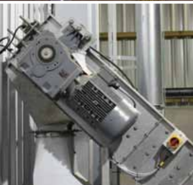
Bevel gear motor provides compact solution.
