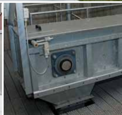
Drive section with outlet and overflow.
