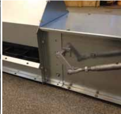
Extension with side inlet and capacity control.
