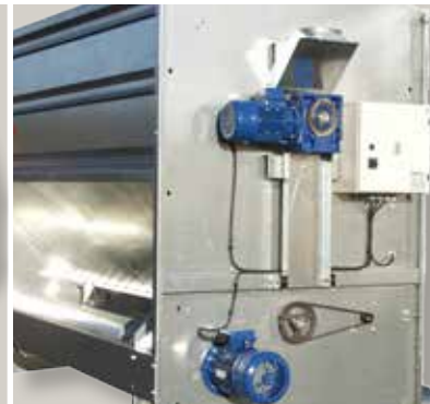
Panel for start/stop of motors in the right order, so blocking of the KDC 4000 is avoided.
