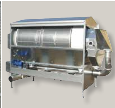
Screen drum with 2 layers of screens. The Inner screen works as scalping screen retaining oversize impurities. The outer screen is a sand screen where small impurities are sorted from the prime product.
