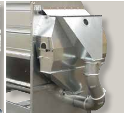
A handle placed on the outside cabinet makes it easy to adjust the aspirator function without any tools.
