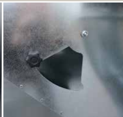
Access door for easy collection of grain sample after cleaning.
