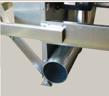
Screenings is conveyed through pipes up to 15m away.
