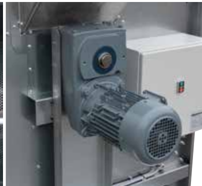
Gear with parallel shaft's makes it easy to turn drum by hand, makes screen change easier.
