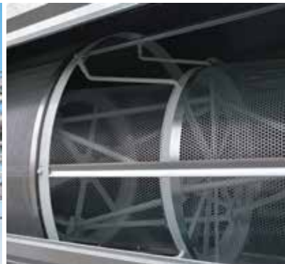
Two layers, one layer for oversize impurities, a second layer for under-size impurities.
