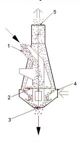
The KFP aspirator models are suitable for capacities above 80 t/h.
