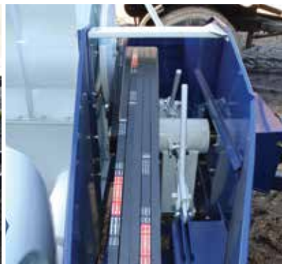
The belts can be tightened without using tools, although tools are required to gain access to the belts.
