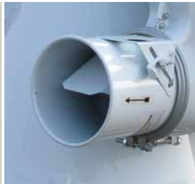
Air regulation for adjusting the suction power of the aspirator.
